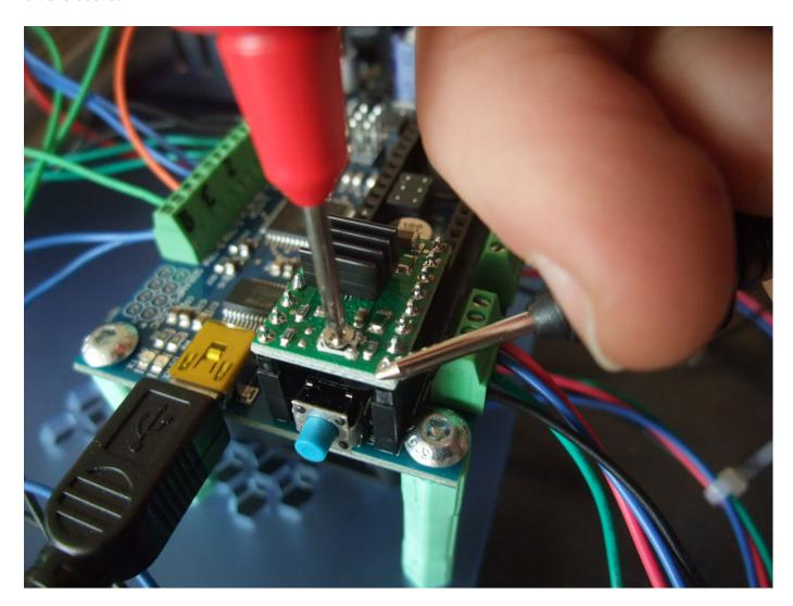
Adjust the pot until you measure, in this example, 0.96V. Now you have your step stick properly adjusted for your motor's current.
