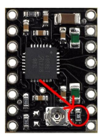
Original Pololu boards have a **0.05**  $\Omega$  resistor while most generic brands use **0.1**  $\Omega$ .
